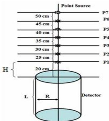
Fig.1: axial motion from the detector.
